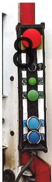
Left: Control box is simple and compact and is also duplicated on both sides of unit. The next step: This Scania/Heil RCV awaits fitment of third Ecoprocess unit to be ordered by Gamathjonustan
