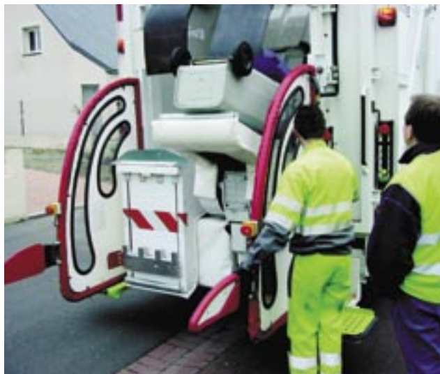
The electric-powered, non-hydraulic, Isbjörn bin-lift in action
